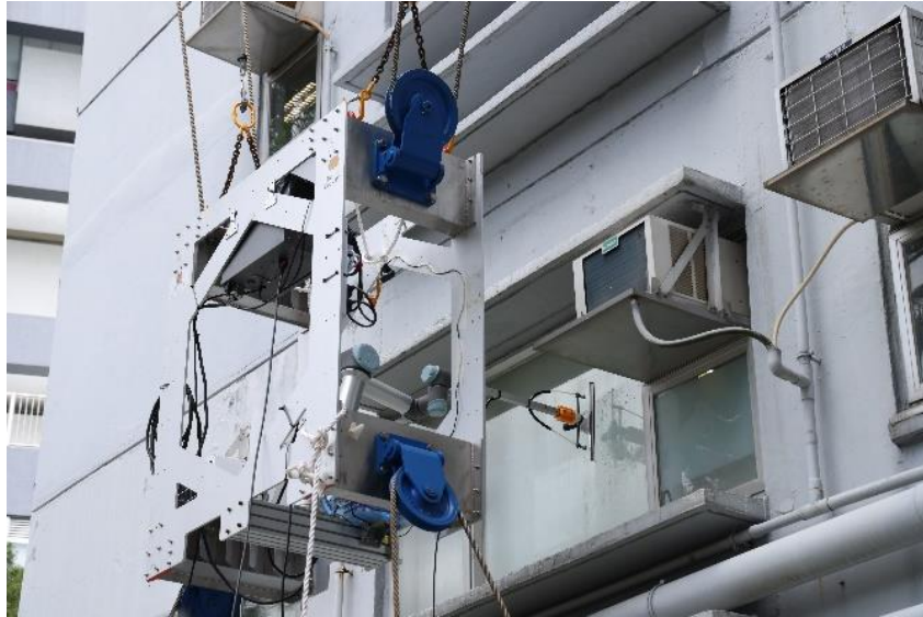
Photo3: The cable-driven robot can mimic human movement to clean building windows and paint facades. The system is expected to replace human wiper and roller-based window cleaning and facade painting works at high-rise buildings, helping to relieve the industry's labour shortages. The photo shows the demonstration of window cleaning.
